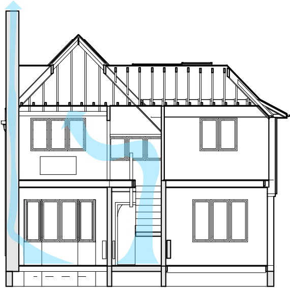
Stack ventilation concept utilising windows and chimney flues
